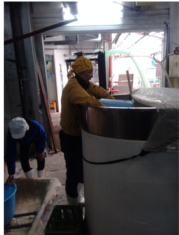
Fig. 5 Steamed and cooled rice was added to unrefined sake . In shikomi , rice and malt are added to yeast mash for further fermentation [15]. To sustain the activeness of the yeasts, rice and malt are not added once but three separate times. One third of the total amount is put each time. Rice is cooled by a machine before being put into a tank. All rice including spilled one is collected during the process. Note. Conventional rice was steamed on the day of the visit. Photo by authors
