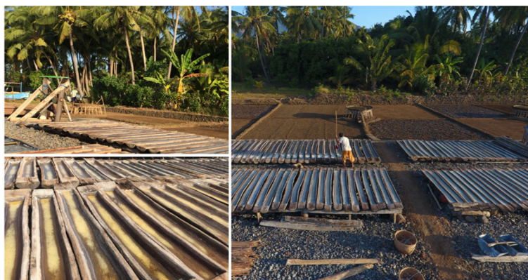
Fig. 1 Palung as the evaporation media to crystallize salt. The media uses old coconut trees and many traditional values are incorporated in the system
